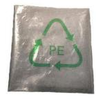
Ethylene is made by *cracking* natural gas or the light fractions of refined crude oil. It is converted to polythene by heat and pressure. A special substance called an *initiator* has to be added to get the *polymerisation reaction* started. Depending on the conditions, the polythene may have upwards of 10 thousand carbon atoms in each long chain molecule.
