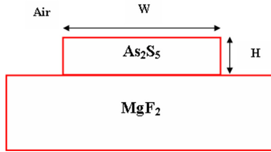
Fig. 1. Cross sectional view of the proposed As 2 S 5 ridge waveguide where the width and the high of the channel are W and H, respectively. Inset simulated fundamental field profile at 2 μm.
