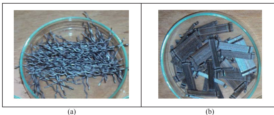
FIGURE 1. Used metal fibers. (a): F1 Corrugated metal fibers, (b): F2 Hooked ends metal fibers.
