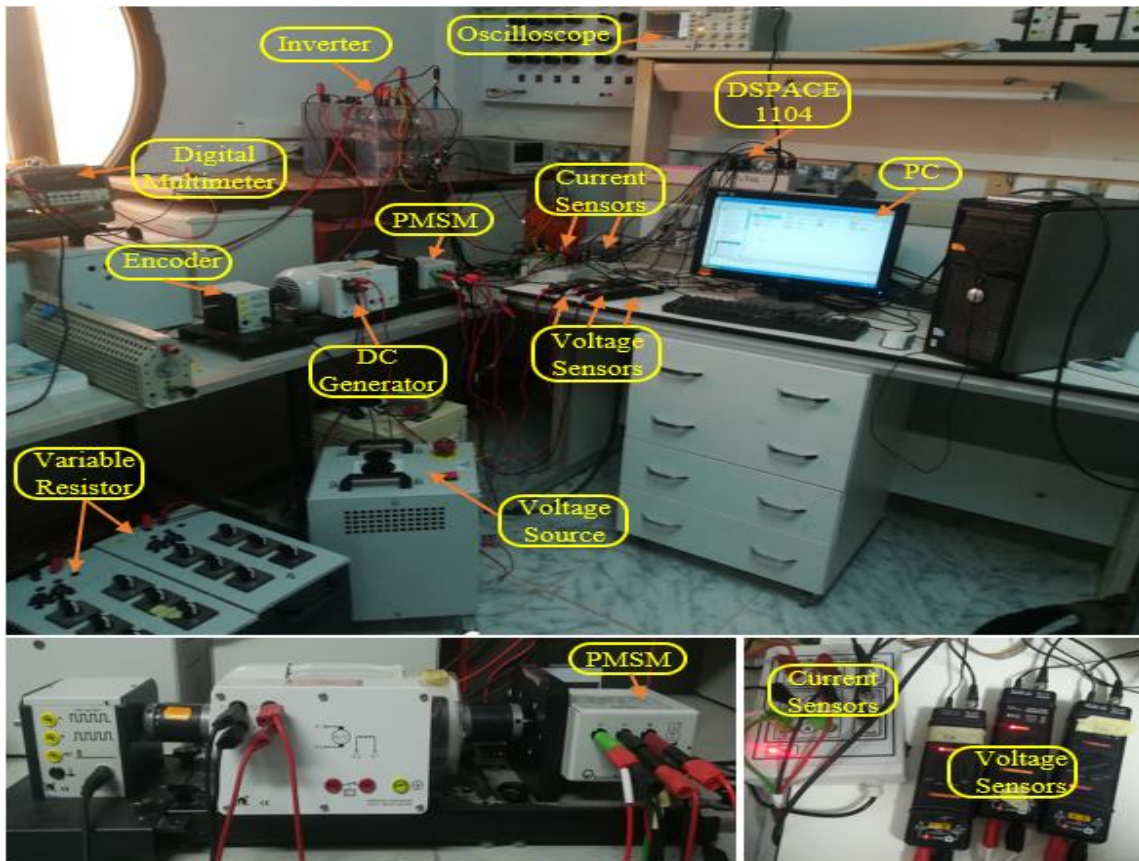
Figure 4.4 Global system experimental test.
