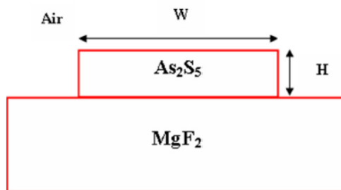
Fig III.1: Cross sectional view of the proposed \text{As}_2\text{S}_5 ridge waveguide where the width and the high of the channel are W and H , respectively [3].
