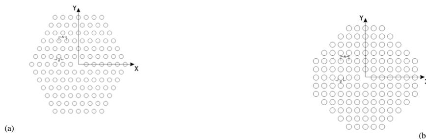
Fig.2. Cross section of V type PCF: the radius of the small and the big holes is  $0.8\mu\text{m}$ ,  $1.2\mu\text{m}$ , respectively
