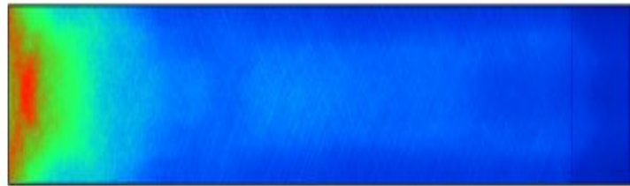
Fig. 4: Absorbed pump distribution along the laser rod
